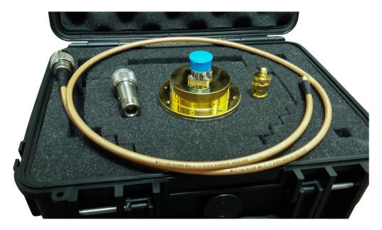
ESDGuns.com CST Current Sensing Transducer for ESD Generator Tip Verification allows the user to take measurements conforming to the requirements of the most recent version of the IEC 61000-4-2 compliance standard up to 4GHz.
