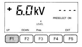
By F5 branch into the preselect counter menu. Press F1 or F2. The counter shows 0000 or 9999 respectively. Continuous operation is switched off.
