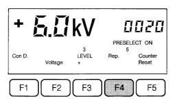
Select the repetition frequency in the basic menu with F4. By F5 branch into the preselect counter menu.
