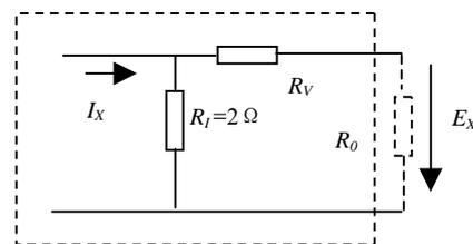
Fig. 2. DC equivalent circuit of the target
