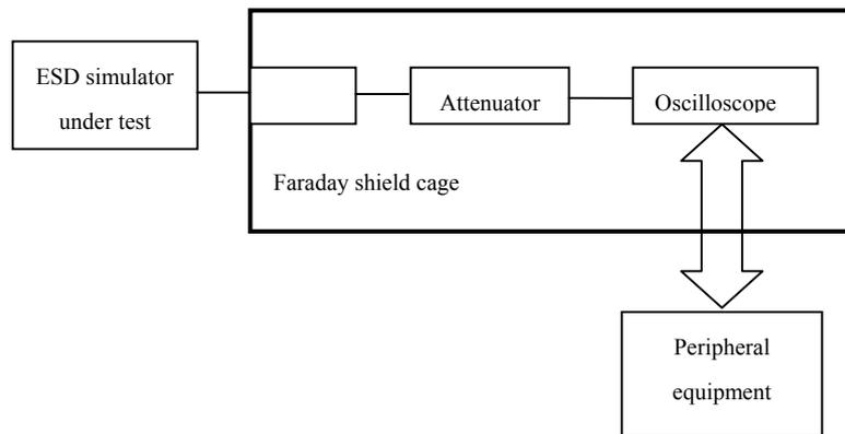
Fig.1. Set up for current waveform calibration subsystem
