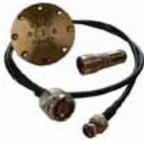
For wave shape verification according to IEC/EN 61000-4-2
