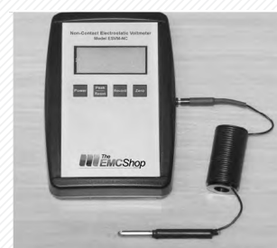
Meter Ground Wire
