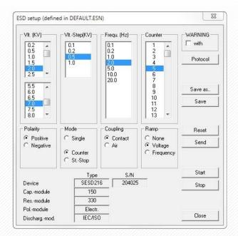
In "READ ONLY" mode, the software registers all operations performed on the ESD generator.
