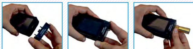
Figure 6. Attaching the sensor module to the ESD Event Meter
