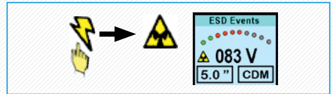
Figure 24. Changing the filter from “True ESD mode” to “All Signal mode”
